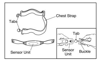
Next, wrap the chest pulse sensor around your chest and attach the other end of the chest strap to the sensor unit. Adjust the length of the chest strap, if necessary. The chest pulse sensor units expected the chest pulse sensor units are chest pulse sensor units.
